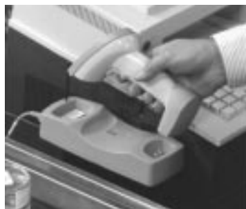
The LS 4071 communicates with the host via the cradle/base station.
